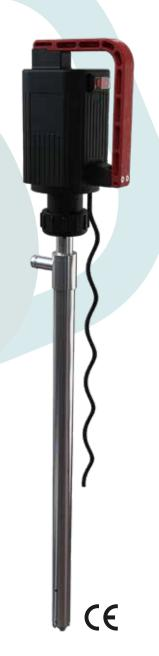
The drum transfer pumps consist of a dip tube, at the end of which the open impeller is fitted. It is secured to the drive shaft, connected to the pump with a ring nut. The operation consists of an impeller integrated with the shaft, connected to the electric or pneumatic motor with a coupling joint. The transfer pumps must be used exclusively vertically and with the pump immersed
