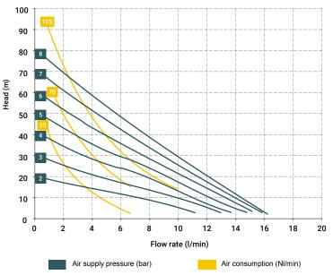
\*The curves and the performances refer to pumps with immersed suction and open delivery outlet, with water at 20°C and vary based on the composition materials.
